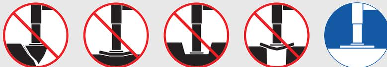
Check that the extra support plates do not bend or sink into the ground.
