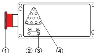
**Lamp indicator for over load (load warning) (4)**
