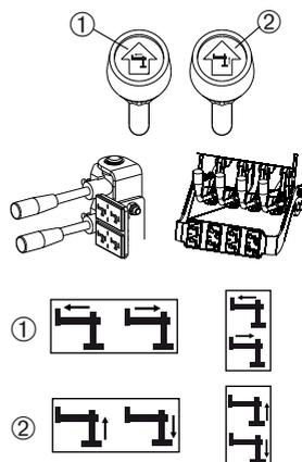
**Operate the stabiliser extensions and stabiliser legs.**
