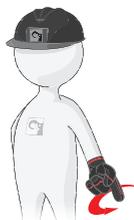
**Stop all crane movements / Hold the load in position**
