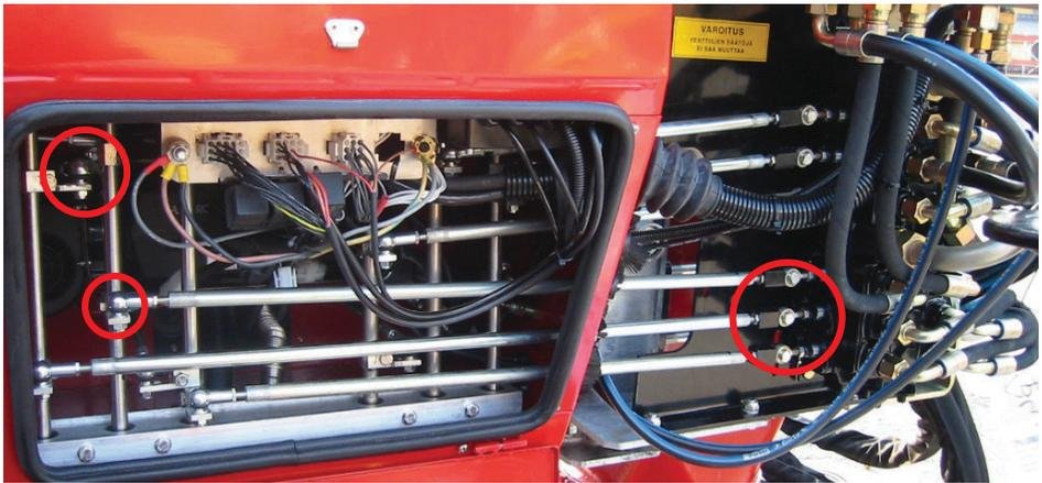
All ball joints must be lubricated monthly. Do not forget the ball joints on the spool ends. The image shows examples of the location of the ball joints.
