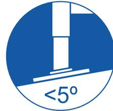
The maximum permitted ground inclination under the stabiliser leg plate is  $5^\circ$ .
