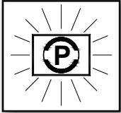
14. Engage the parking brake when the container rear end is lifted from the ground.
