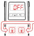
Press both top buttons for 5 seconds to exit the software and return back to normal operation.
