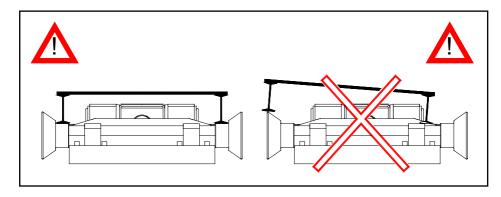
When loading and unloading a container, be sure that it is running in line between the rear rollers
