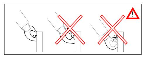
Before picking up the container, the gripping bar of the container must be properly inside the lifting hook. In this way you prevent the container from falling. The situation must be checked by lifting the container approx. 3.9 in (10 cm) and after that checking physically and visually that the container gripping bar is inside the lifting hook.
