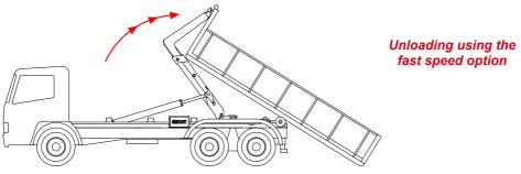
The fast speed option is integrated with the load holding valve, enabling an optimized oil flow when driving the main cylinders outwards. The load holding valve maintains a controlled movement along the entire length of the cylinder.
