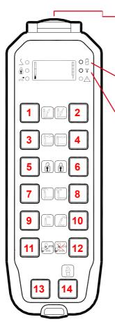
Activate the radio controller by turning the **ON / OFF** switch.
