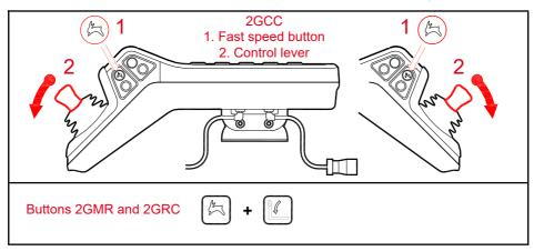
You can use the fast container lowering feature to lower the container faster than normal speed. The speed of the fast lowering is affected by the weight of the empty container and the temperature of the oil; at cold temperatures the speed decreases.
