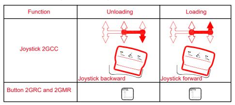
Moving the joystick backward will activate the unloading movement, which is automatically followed by the following operations:
