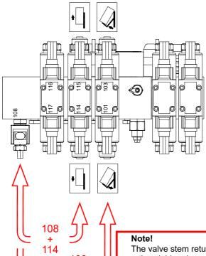
If a failure happens in the electric system of the device, the device may be restored to its normal state, by operating the control valve manually:
