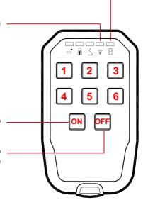
The XR equipment function\*) is activated by simultaneously pressing the **ON** switch and the button for the **function to be activated** (ON+1, ON+2, ON+3, ON+4, ON+5 ja ON+6).
