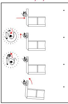
Reverse the vehicle so that the hook is below the gripping bar.
