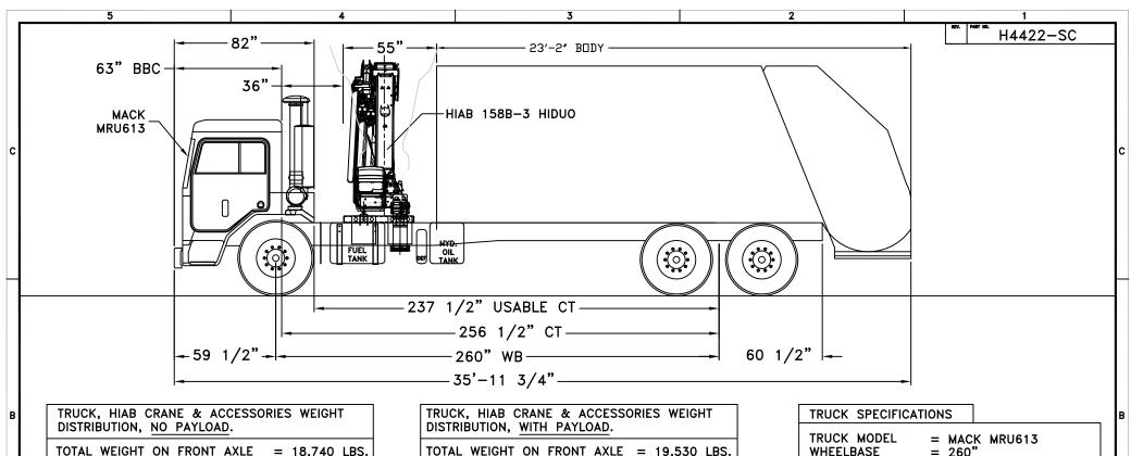
TOTAL WEIGHT ON FRONT AXLE = 18,740 LBS. TOTAL WEIGHT ON TANDEM AXLE = 24,240 LBS. FRONT AXLE WT. PERCENTAGE = 44 % TANDEM AXLE WT. PERCENTAGE = 56 % GROSS VEHICLE WEIGHT = 42.980 LBS.
