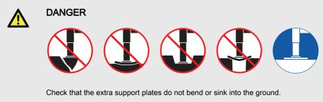
Do not lower the stabiliser legs on the edge of an embankment, soft ground, hollows, etc... Lower the stabiliser legs only on to a flat, firm and stable surface.
