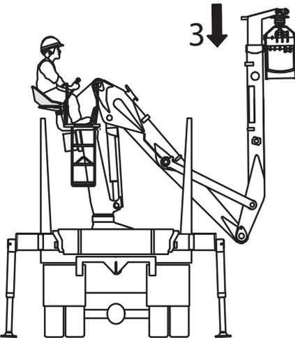
3. Retract the hydraulic extensions until the grapple is locked in the support.
