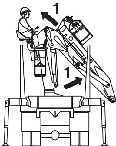
1. Drive the extensions out until it is released from the catch. Then, operate the 1st boom 1-1,5m out from the column.
