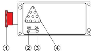
**Lamp indicator for over load (load warning) (4)**
