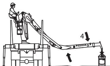
4. Press the grapple against the ground and straighten the 2nd boom.
