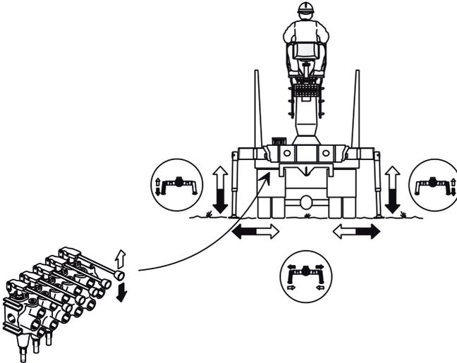
The crane is equipped with a stabiliser control valve. The valve can be operated with the levers on the valve and from the high seat [option].
