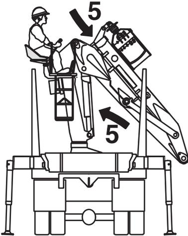
5. Retract the extensions until it is locked by the catch. Slowly operate the 1st boom against the column.
