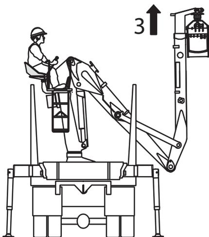
3. Extend the hydraulic extension until the grapple is released from the support hook.
