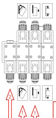
If a failure happens in the electric system of the device, the device may be restored to its normal state, by operating the control valve manually:
