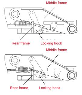
A mechanically actuated tipping lock is located between the rear frame and middle frame, consisting of a hook that grips around the locking lug. The hooks are fully exposed when the hookarm is completely retracted. The hooks are locked automatically when the telescopic hookarm is extended forwards by more than 3.9 in (100 mm). During tipping, the middle frame is locked to the rear frame by the tipping lock. The lock is automatically operated when the hookarm is activated.
