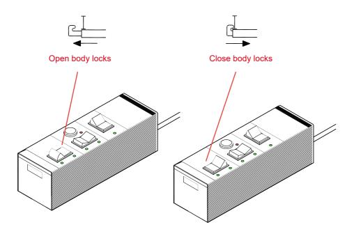
The body locks open when the user presses the back of the boidy lock rocker switch and close when pressing the front part.
