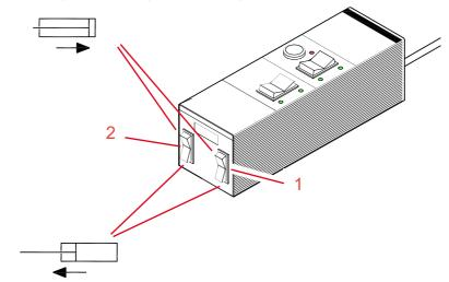
Drive the cylinder of the hydraulic auxiliary equipment out
