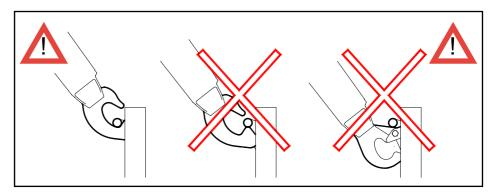
Before picking up the container, the gripping bar of the container must be properly inside the lifting hook. In this way you prevent the container from falling. The situation must be checked by lifting the container approx. 3.9 in (10 cm) and after that checking physically and visually that the container gripping bar is inside the lifting hook.
