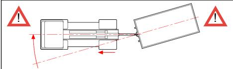
When loading, the container must be placed in line with the driving direction of the truck.
