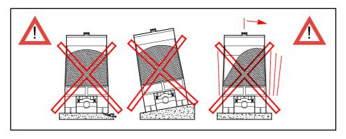
Never load, unload or tip a container when the load is heavier to one side or the ground is sloping.
