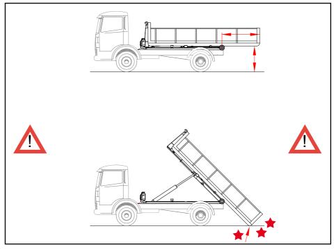
In very cold weather the load might freeze tight on the container. In that case it must be freed before tipping. Note that the load might come out in large chunks!
