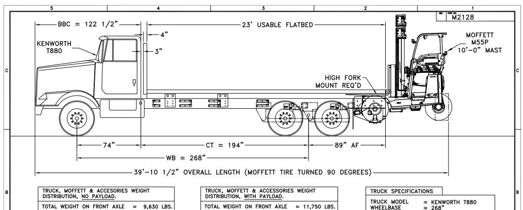
TOTAL WEIGHT ON FRONT AXLE = 9.630 LBS. TOTAL WEIGHT ON TANDEM AXLE = 24,540 LBS. FRONT AXLE WT. PERCENTAGE TANDEM AXLE WT. PERCENTAGE = 72 % GROSS VEHICLE WEIGHT = 34.170 LBS
