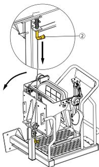
1. Pull lever (2) to unfold the seat.
