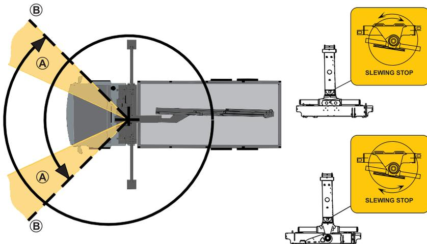
2. Slew the crane slowly in each direction to the slewing stop (B).
