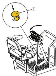
4. Press the pedal (3) to adjust the distance to the controller.
