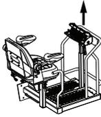
2. Remove the controller from its holder.
