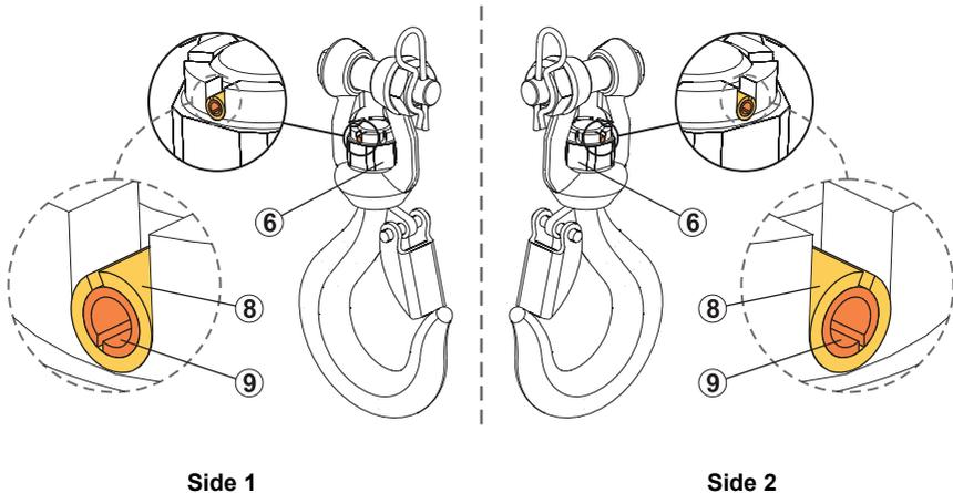
The two Spring/Roll pins (8) and (9) should be in place and nearly flush with the outer edge of the hook nut (6) on both sides. (See the pictures **Side 1** and **Side 2**).
