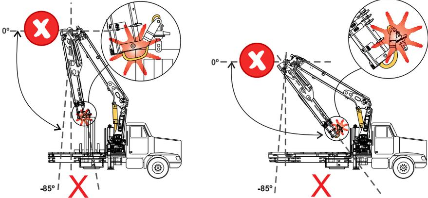
To avoid possible collision between the boom tip and rotator/hoses:
