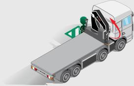
1. If the stabiliser system is manually controlled, push button
