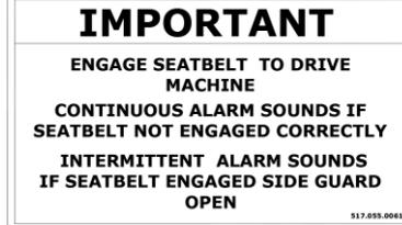
**Note:** The machine is fitted with an interlocking seatbelt. The machine will not drive unless the seatbelt is engaged. If seat presence is fitted an alarm will sound if correct sequence is not followed.
