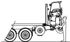
10. With the engine running and the backup alarm audible, the buttons on the handset are now live.
