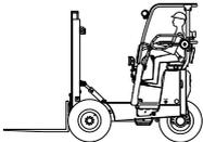
7. Extend the mast fully until the load is directly above the landing area or trailer.
