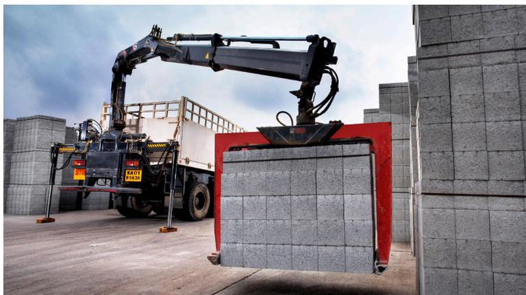
It is very important to understand that your chassis RBM (Rated Bending Moment) specs will play a role in determining the size of crane that a chassis can handle. Therefore, RBM specs must be selected correctly when choosing a truck. In all of these areas of questions, Hiab's product support team can assist you to determine feasibility.
