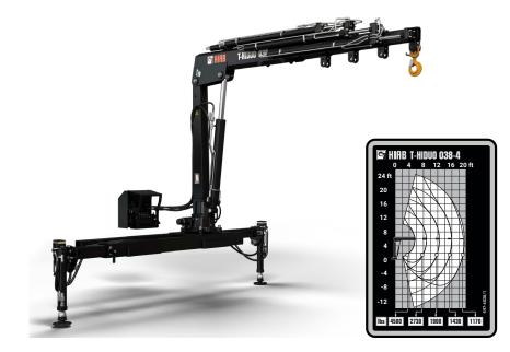
For utility trucks involved in moderately heavy loading operations, the HIAB T-038 range is the perfect match. Available with two, three or four hydraulic extensions, it has a lifting capacity of 4,500 lbs at close range, plus an outreach of up to 22'. These characteristics make it ideal for handling loads such as heavy gardening equipment, medium-size machinery and building materials.
