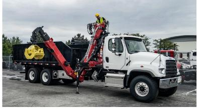
It's crucial that the truck frame can handle the movement, twisting and stress of the loader when operating at maximum outreach and lifting capacity. It is very important to understand the chassis Rated Bending Moment or RBM. RBM specs play a role in determining the size of the loader that a chassis can handle. Therefore, RBM specs must be selected correctly when choosing a truck. In all of these areas of question, Hiab's product support team can and will assist you in determining feasibility.
