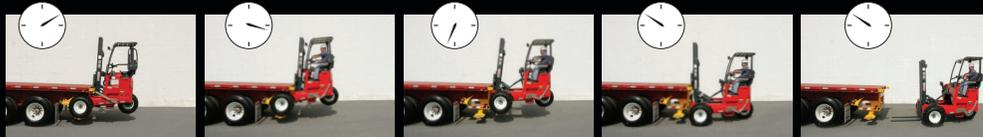
In less than a minute, the Moffett can mount or dismount a truck or trailer and be ready for work.
