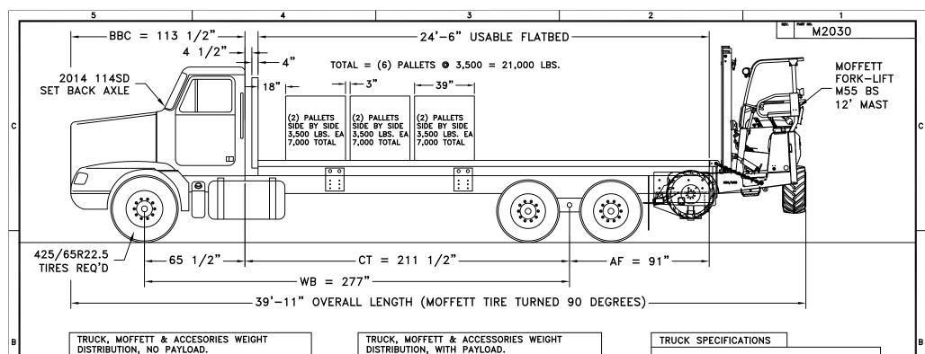
TOTAL WEIGHT ON FRONT AXLE = 9.700 LBS. TOTAL WEIGHT ON TANDEM AXLE = 22,220 LBS. FRONT AXLE WT. PERCENTAGE = 30 % TANDEM AXLE WT. PERCENTAGE = 70 % GROSS VEHICLE WEIGHT = 31.920 LBS.
